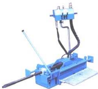
Grundopit - technique de branchement, type standard: DN ≤ 110, 50 m type Power: DN ≤ 160, 80 m
